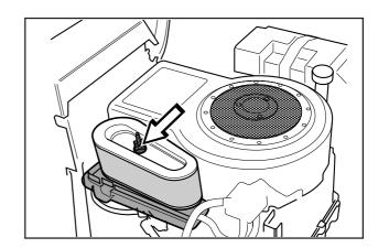
**4.** Pull off the foam plastic pre-filter from the paper filter and wash clean in mild detergent.
